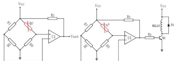
This is an ideal circuit for applications that require on-off switching at a specified force.
